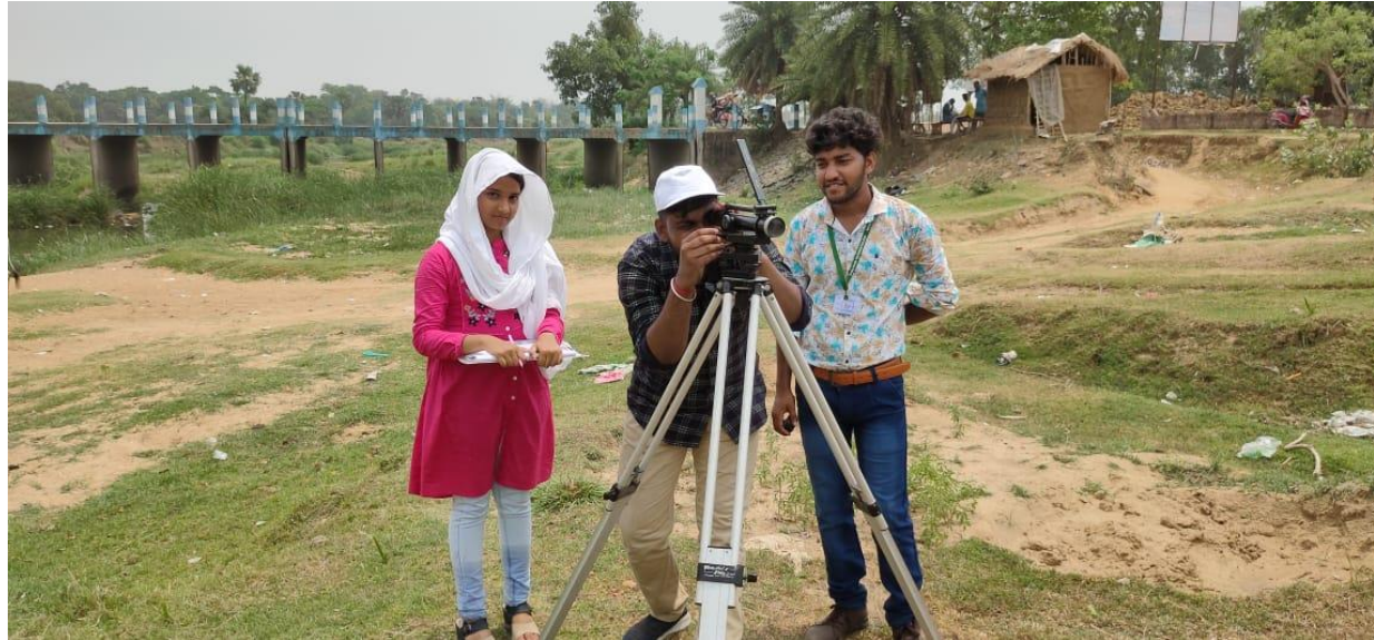
Dumpy Level Survey on Right Bank of River 'Kopai'
